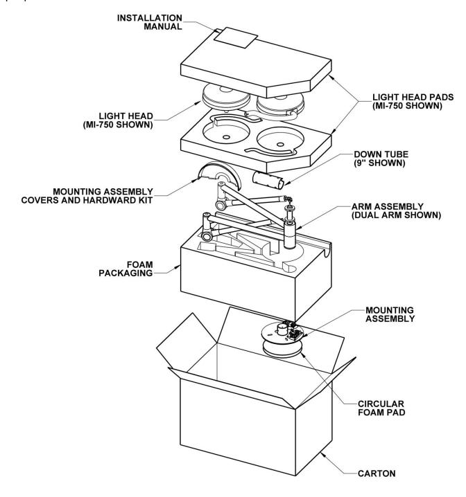
Figure 6: Packing Contents (Dual MI-750 shown)
