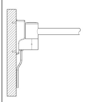
Figure 16: Wall mounting with load anchor or stud-anchor
