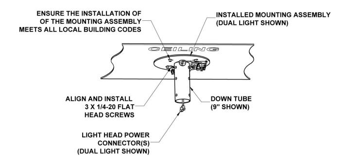
**Figure 7: Mounting Plate Installation**
