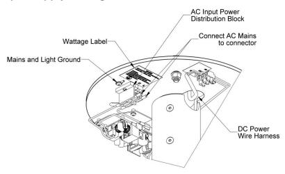
Figure 11: Connecting AC Mains
