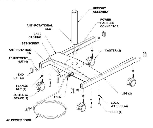
Figure 19: Floor Stand Base Installation
