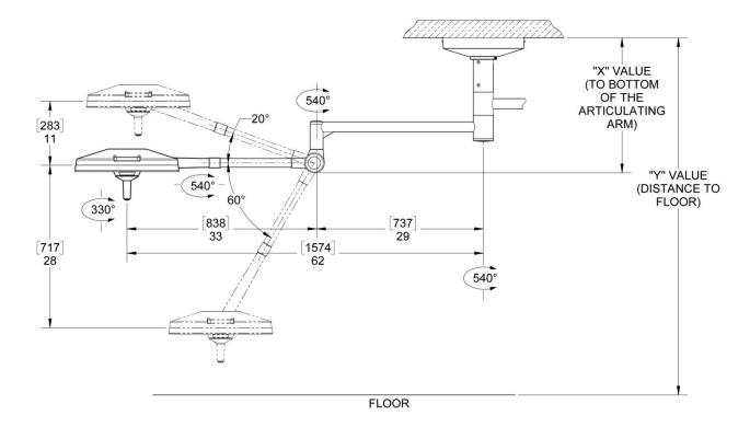
Figure 2: Ceiling Rod Calculation for Dual Ceiling Mount
