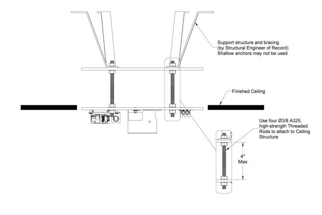
Figure 3: Recommended Ceiling Structure Construction
