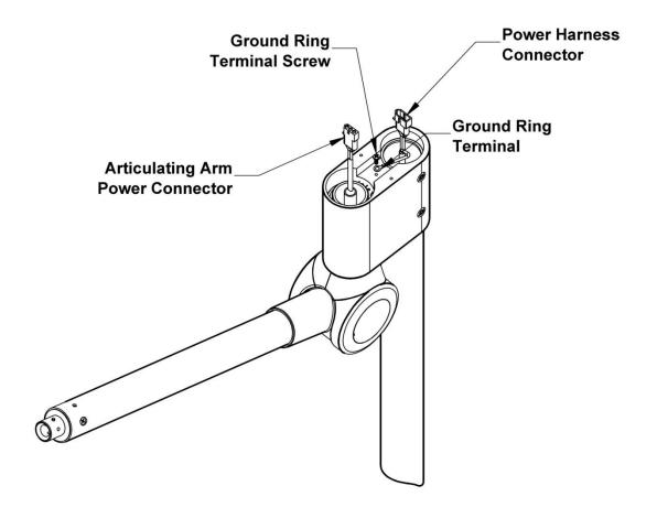
Figure 22: Articulating Arm Electrical Connection
