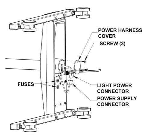
Figure 20: Floor Stand Electrical Connection
