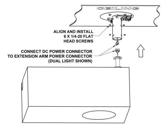
Figure 8: Installing the Arm Assembly
