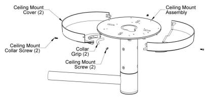
Figure 12: Installing the Ceiling Mount Covers
