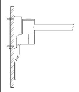
Figure 17: Wall mounting with Back-Plate
