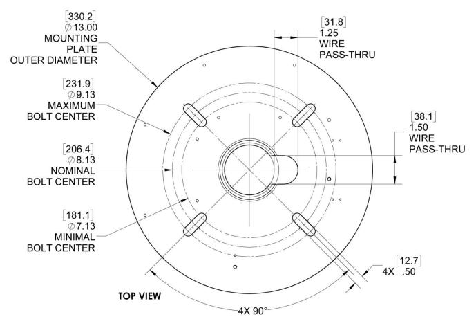
**Figure 4: Mounting Dimensions for Ceiling Mount Assembly**
