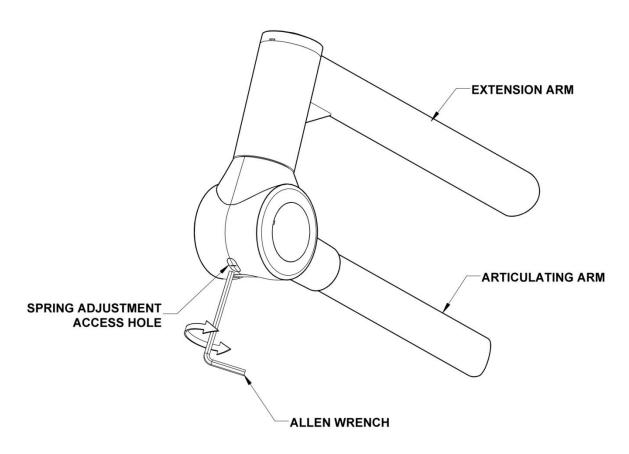
Figure 23: Adjusting the Articulating Arm
