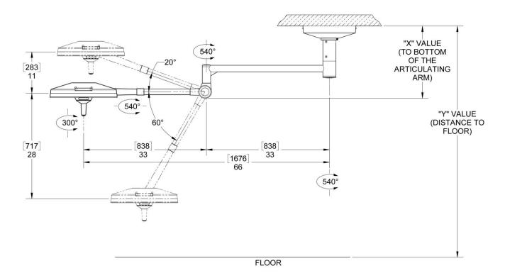
Figure 1: Ceiling Rod Calculation for Single Ceiling Mount
