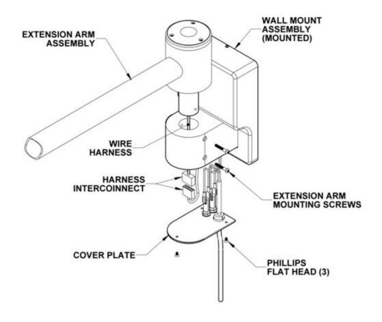
Figure 15: Extension Arm Mounting on Wall Bracket
