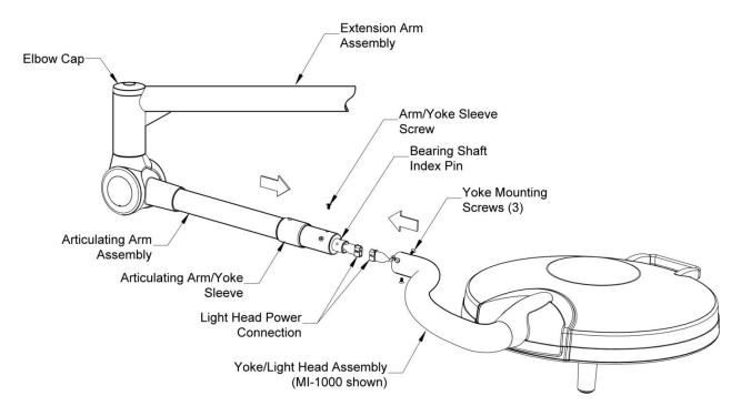
Figure 10: Installing the Light Head
