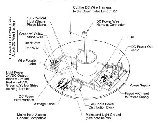
Figure 5: Arm Cable Termination
